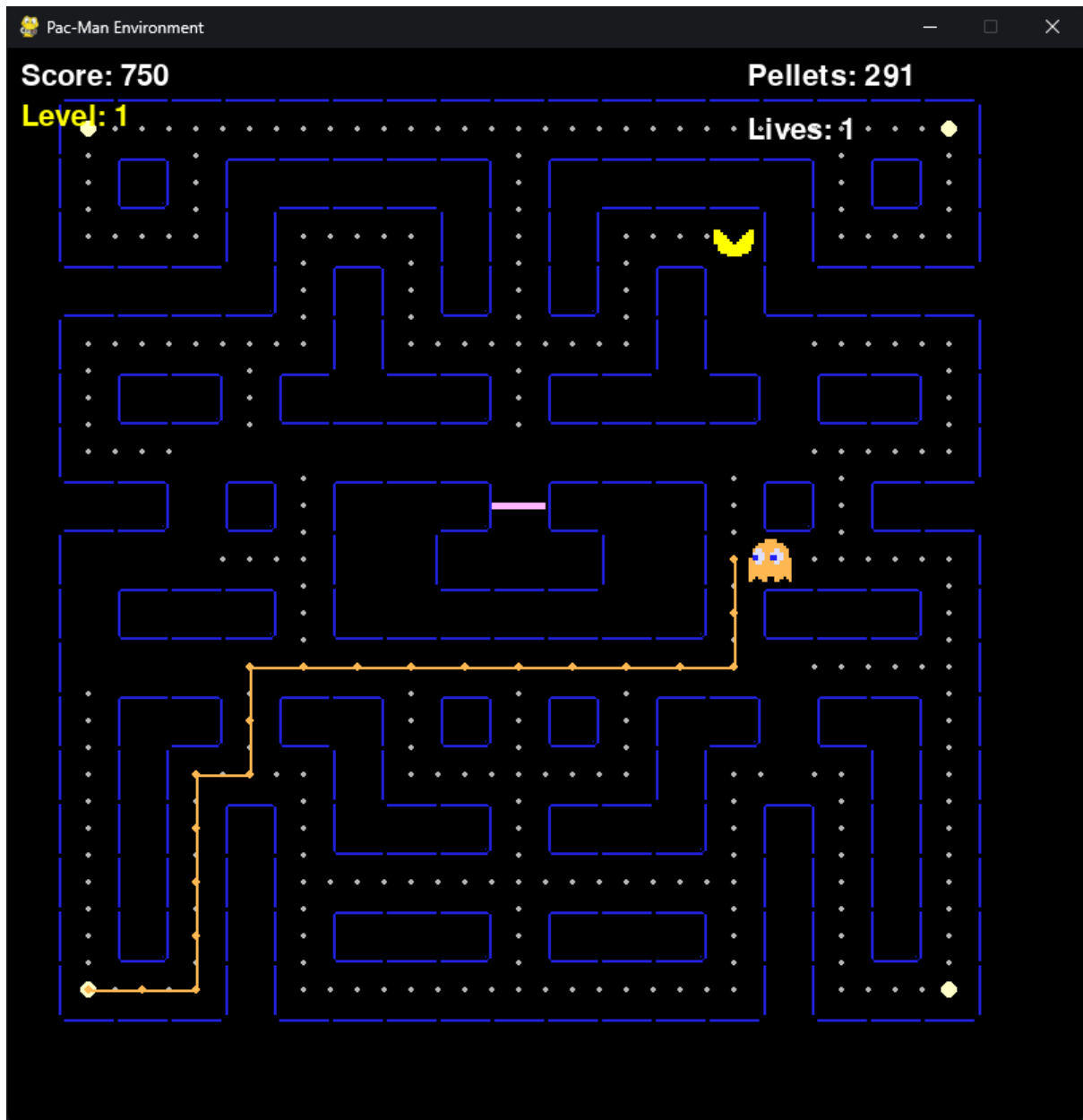
Figure 3.11 Clyde retreating to its corner scatter position when within 8 tiles of Pac-Man
